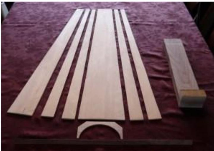
The large piece in the center is the soundboard, with two side pieces to the right, two side pieces and the back to the left, the bottom brace and wood for bottom trim below, and the pieces that would be shaped into the neck and peg box to the extreme right.
